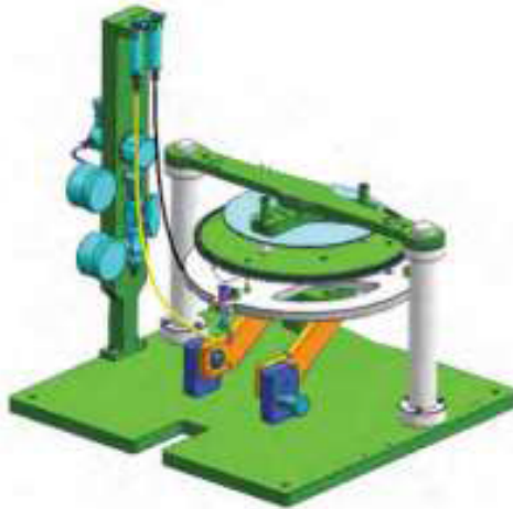
Cable routing for the sensor assembly
