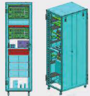
Design concepts of E-cabinet and its components for a test stand
